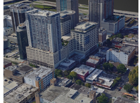
3D textured mesh .ply, .fbx, .dxf, .obj, .pdf Level-of-detail mesh in .osgb, .slpk
